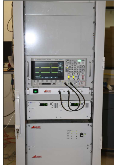
Cabinet System Dual Channel Puls Unit set with 4-Channel Measurement System
